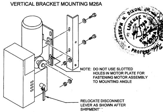
NOTE: Motor assembly is shipped ready to be installed with mounting members and brackets pre-drilled, all necessary hardware and correct length of roller chain required. Follow these instructions carefully for correct mounting of motor operator.
